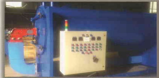
Oil Fired Thermic Fired Heater (Duo Block Burner)
